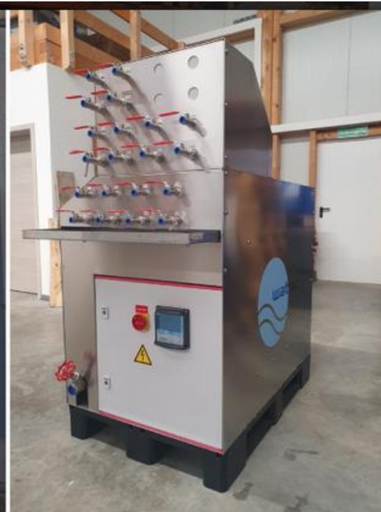
picture left: Operating display of the Dreyproper 4.2 for controlling and monitoring the cleaning process in the cooling channels of injection molding tools.
